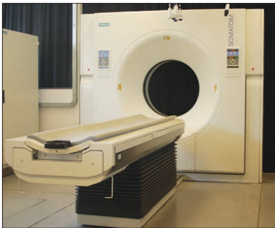
4.23 Multi-slice helical computed tomography scanner, with the patient couch in the foreground and gantry at the back.
