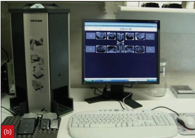
4.8 (a) Phosphor plates within disposable plastic sleeves. (b) Scanning (laser reader) machine used to transfer latent images on to a computer.
