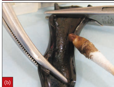
13.28 (a) Debris emerging from an ultrasonic handpiece. (b) Biofilm inside a cut plastic tube carrying water to an ultrasonic scaler.
